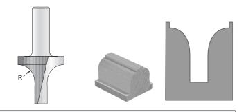
Plunge Type Rounding Over Bits, 2 Flutes with Boring Point (Corner Round)
