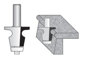
Undermount Profile Bowl Bit, with Bearing, 2 Flutes Part Cutting Cutting Radius Bevel Shank Overall Number Dia Length Dia Length
