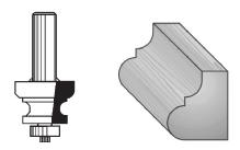
Cutting Radius Shank Part Cutting **Overall** Number Dia Length 1&2Dia Length LR94084 13/16" 19/32" 5/64" 1/2"2 - 1/2" LR94085 1-1/4" 7/8" 5/32' 1/2"2-3/4" LR94086 1-9/16" 1-3/16" 7/32" 1/2" 3-1/16"
